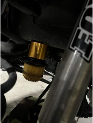
Remove the factory bump stop by pulling it out of its mount. Remove the mount from the frame by pulling it out of its mount. Install the bump stop spacer and factory bump stop mount to the frame using an M8  $\times$  70 mm bolt and washer. Torque to 5 ft-lbs. Install the bump stop to the factory mount by pressing it back into place.
