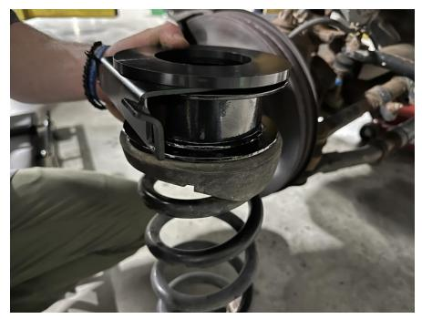
Make sure not to over-extend the ABS, brake lines, and vent tube. Install the urethane isolator, shock reservoir mount, spring spacer, and then factory rubber isolator onto the spring. Raise the axle enough to hold the spring assembly in place. The assembly should look as picture above.
