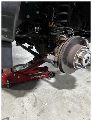
Raise the front of the vehicle and support it with safety jack stands at each frame rail behind the lower control arms. Support the axle with a suitable jack.
