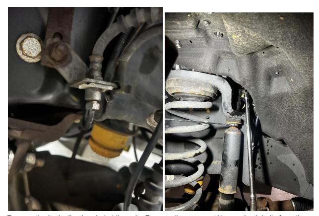
Remove the brake line bracket at the axle. Remove the upper and lower shock bolts from the axle mount. Remove the sway bar from the frame. Lower the axle enough to remove the front springs.
