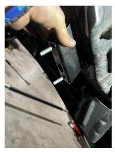
Install the sway bar drops to the frame using factory hardware. Torque to 35 ft-lbs. Install the sway bar to the sway bar drops using the 7/16" x 1 1/2" bolts, washers, and nuts. Torque to 35 ft-lbs.
