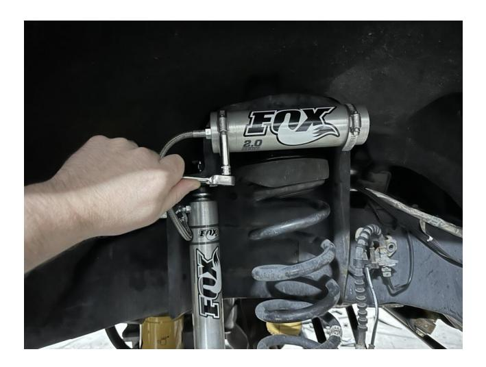
Install the shocks with factory hardware. Mount the reservoir with the Fox clamps on to the mount. Install the rear shocks if included. Torque shock hardware to 35 lb-ft.
