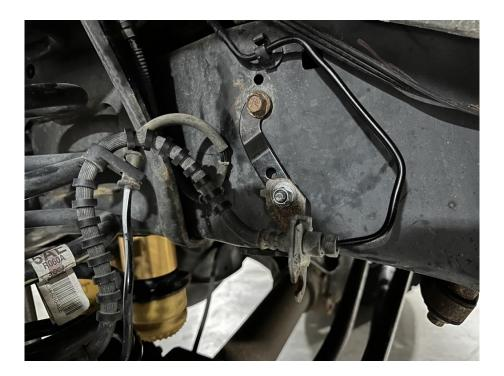
Reattach the factory brake line bracket at the axle using factory hardware. Torque to 5 ft-lbs. 2011 - 2016 front brake line: Install the brake line drop bracket to the frame using the factory hardware. Torque to 5 ft-lbs. Note: The brackets look like the factory brackets, except the locating flat is 180 degrees off. Install the brake line block using the factory clip. Reconnect the ABS line. Do not clip back to the fender liner.
