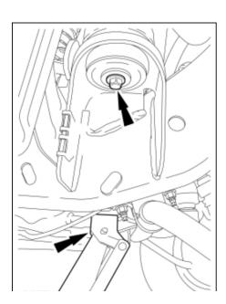
2. Remove all of the other bolts. It may be necessary to have someone hold the cage nuts from the top. You will need to pull the carpet back to get access to the inside cab plugs. You will need to remove plugs and hold the cage nuts with a socket.
