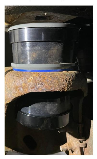
5. After Installing the mounts tighten down with the new provided bolts and washers to 76 Lb-Ft (Ford TQ amount).
