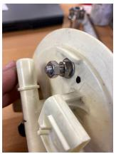
2. Find a suitable location drill and Install -8 feed hose bulkhead into the top of the pump hat as shown. Make sure to check house routing so it doesn't kink. The Nylon hose will require heat (Boil in water) to expand and go over the barb.
