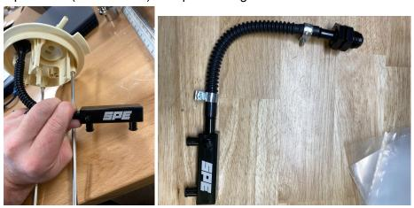
3. Once the main connections are made connect the small siphon hose from the manifold to the bucket. It will need to be cut to length. Make sure when installing the manifold to the pump outlets to keep it as close as possible to the pumps.
