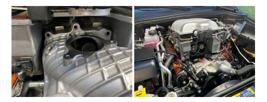
Using a 1" allen socket or bolt and SPE holding block remove the factory blower pulley. Install the SPE Hub onto the blower shaft, torque to 75 LB FT Using the supplied hardened hub socket as shown. Blue Loctite is recommended.
