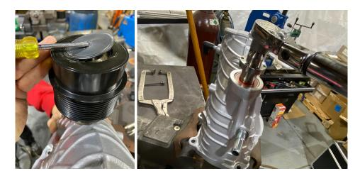
3. Install the the blower pulley and included allen bolts torque them to 100 IN LB
