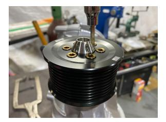
4. In reverse of the disassembly procedure Install the blower shaft and pulley assembly into the blower case and remount blower assembly.
