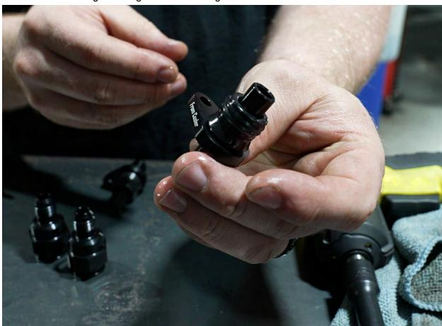
8. Install the spring clips on to the new cooler quick connect adapters.
