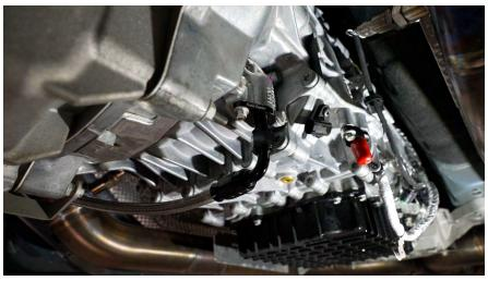
11. Route the second hose in a similar fashion, making sure to go over the sway bar. Connect the 90 degree hose ends to the cooler and transmission.
