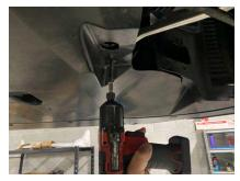
2. Remove the 8mm bolts that attach the factory lines to the transmission.
