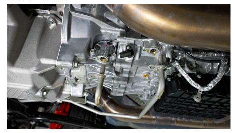
7. Install the seals onto the transmission adapters as shown. Then, install them into the transmission, matching the from cooler fitting to the from cooler casting on the side of the case above the fitting bore. Tighten with the original 8mm bolts.
