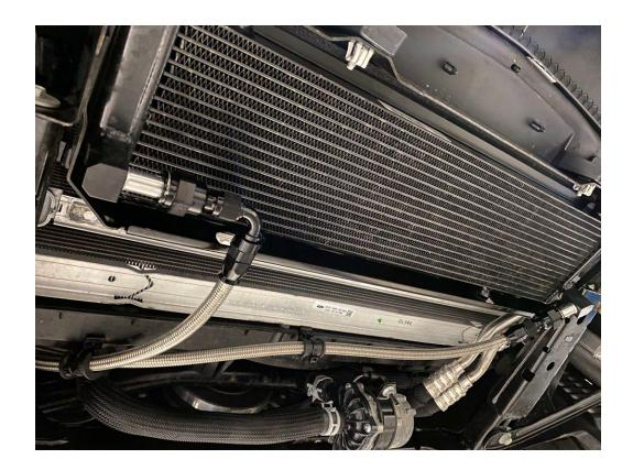
13. Now that the line kit is installed follow the Ford fill procedure to set the proper fluid level.
