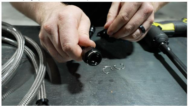
9. Remove the rubber/plastic guides and isolators from the old lines. They will be reused at similar points on the new lines. This will aid in routing and positioning.
