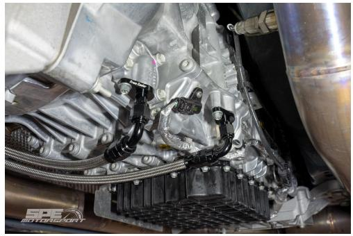
12. Install the Isolators and line clips similar to factory positions (pictures below). Check routing and make sure all fittings are snug.
