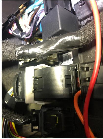
Pull out the harness push clip, and install the metal tab coming off of the module underneath of it to secure in place.
