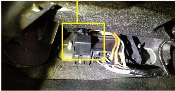
Once all connections are made, you can attach the device to the top of the module with the supplied adhesive patch.
