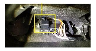
Once all connections are made, you can attach the device to the top of the module with the supplied adhesive patch.
