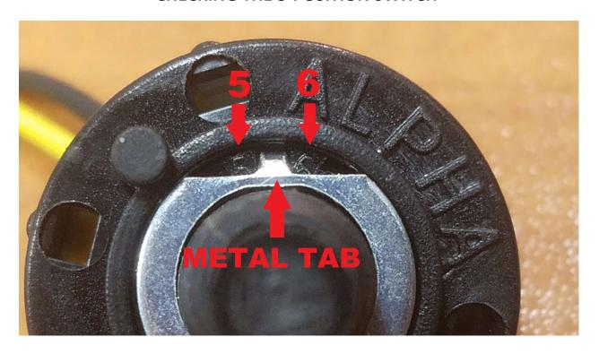
Remove the switch and inspect the location of the metal tab.
