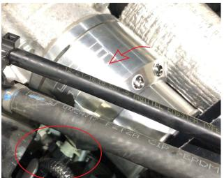
7. Install the supplied clamps onto the charge hose loosely so they can be adjusted and moved. Install the hose onto the intercooler and then the throttle body adapter.
