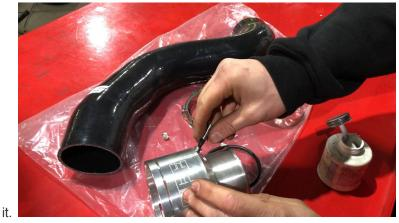
5. After assembling the adapter lube the o-ring with a dielectric grease or equivalent. Install the adapter onto the throttle body make sure the o-ring starts on even, push until you hear a click.
