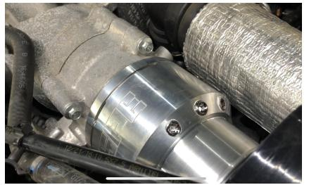
6. Rotate the adapter so the CAC sensor hole is accessible. Install the sensor as factory, twisting clockwise. Re-route the electrical connector and wiring making sure it clears and doesn't snag.
