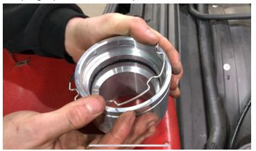
4. Install the supplied plug fittings into the adapter. At this point if you are planning to use an injectable or a port for reference (boost gauge/sensor, temp etc) this would be the time to install
