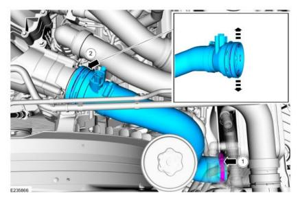
3. Install the supplied o-ring into the new throttle body adapter. You will also be installing/reusing the spring clip out of the old adapter.
