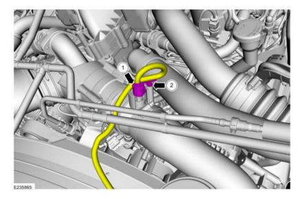
2. Loosen the T-bolt clamp at the outlet of the intercooler. Release the clip and remove the CAC outlet pipe assembly.
