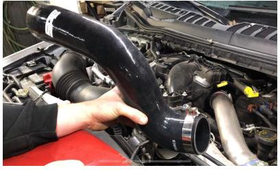
8. Tighten the T-bolt clamps after adjusting the pipe for best fitment.
