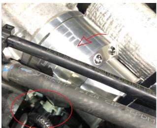
8. Install the supplied clamps onto the charge hose loosely so they can be adjusted and moved. Install the hose onto the intercooler and then the throttle body adapter.
