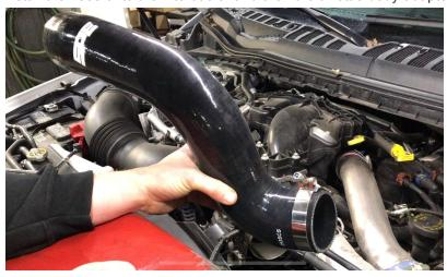
9. Tighten the T-bolt clamps after adjusting the pipe for best fitment.
