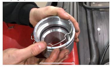
5. Install the supplied plug fittings into the adapter. At this point if you are planning to use an injectable or a port for reference (boost gauge/sensor, temp etc) this would be the time to install
