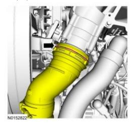
2. Loosen the T-bolt clamps at the top of the coupler and at the outlet of the intercooler.
