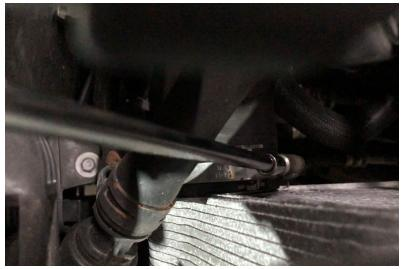
10. After completing your install we recommend driving the truck for a day or two allowing for heat cycles, then going over your hose clamps to make sure they are nice and tight.
