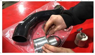
6. After assembling the adapter lube the o-ring with a dielectric grease or equivalent. Install the adapter onto the throttle body make sure the o-ring starts on even, push until you hear a click.
