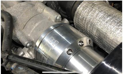
7. Rotate the adapter so the CAC sensor hole is accessible. Install the sensor as factory, twisting clockwise. Re-route the electrical connector and wiring making sure it clears and doesn't snag.
