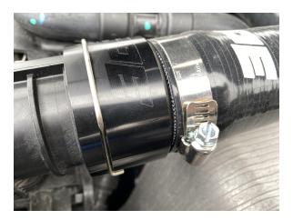
3. Slide the included scroll clamps on the new silicone radiator hose and install the hose on to the adapter. Move the clamps into position and tighten.
