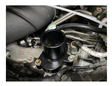
2. Lube and install the o-ring into the billet radiator adapter. Next, install the spring clip into the adapter's grooves with the SPE facing the hood. Press the adapter on to the radiator.
