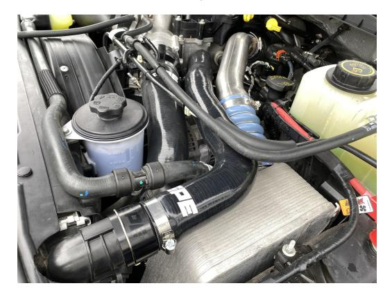
\*\*Note Some 2020 and 2021 model year trucks may have a T assembly in the radiator hose. If your truck has it, trim roughly 2" from the hose and install it in the factory location. You can use the clamps as a guide to trim the hose. Place the clamp where you would like to cut. Using a razor blade, cut around the hose using the edge of the clamp as a guide.
