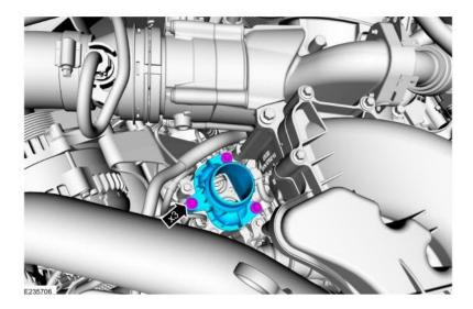
**NOTE**: During installation verify the thermostat vent hole is at the 12 o'clock position.
