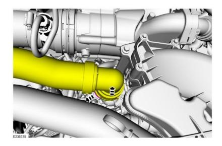
3. Remove the bolts and the coolant outlet connection.
