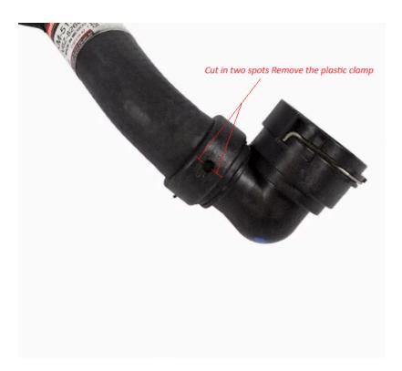
5. Install the ends into the new hose and install on onto the truck make sure the spring clips are secure in their groove. Once you're happy with the orientation, use the provided scroll clamps and tighten them. Install the plastic hose guides and the -6AN ORB plug into the billet hose joint. This can be used the next time you service the cooling system being it's the lowest point to drain your coolant from. This will make the likelihood of taking a bath when removing the lower hose zero.
