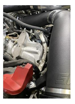
6. Prepare the coldside intercooler pipe for installation slide on the included straight and 90 degree coupler. Install the charge temp sensor into the billet bung.
