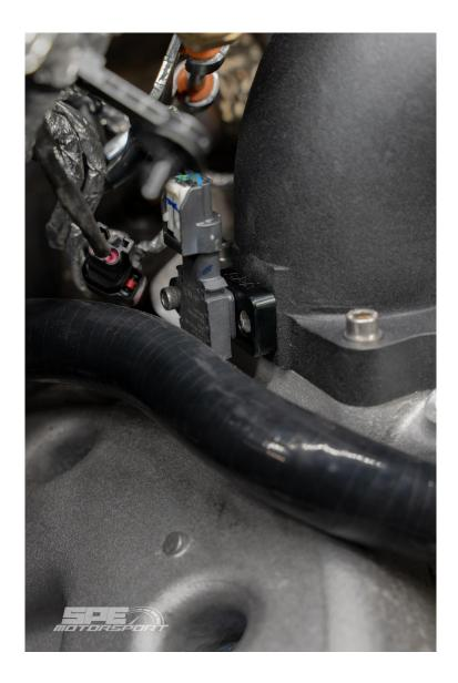
Install the intake manifold Y with the included allen bolts and washers (5mm hex drive). Install them finger tight. Install the dipstick tube bracket. It uses the rear driver side bolt closest to the outside of the vehicle. Use the factory bolt that attaches the trans and oil tubes together. Once everything is attached, tighten all the bolts.
