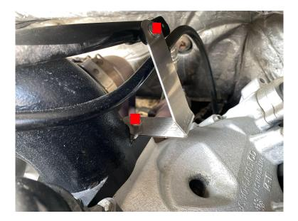
4. Remove the power steering reservoir bolt and pull up on the reservoir. Turn it counter clockwise and reinstall without sliding it back into the guides in the fan shroud. This allows extra clearance for the cold side pipe.
