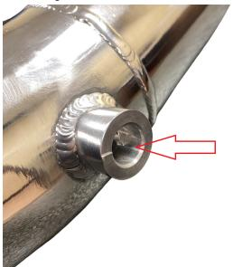
7. Install the cold side intercooler pipe as shown. Connect the temperature sensor carefully routing the wiring. Make sure all clamps are tight and nothing is rubbing. After driving, check the T bolt clamps again.
