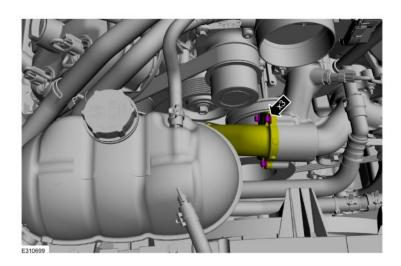
**NOTE:** During installation verify the thermostat vent hole is at the 12 o'clock position. Remove the thermostat. Inspect the O-ring seal and replace it if necessary. During installation, make sure the coolant outlet connection is fully seated on the thermostat housing before tightening the bolts.
