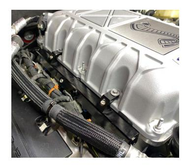
10. Cut/modify the plastic hose guide rail for the driver side as shown.
