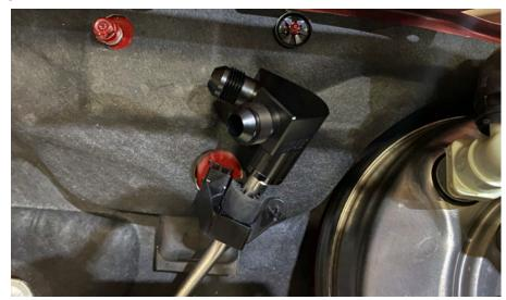
9. Install your injectors into the fuel rails. Place the fuel rails on the blower with the hoses loosely attached to them. Then attach the hoses to the fuel Y once routed correctly. Driver side hose has two 90 degree hose ends. Passenger side hose will have the 45 hose end facing the Y adapter with the 90 hose end on the rail. Tighten all bolts and hoses. Install fuel pressure sensor.
