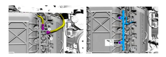
8. Install the Y manifold adapter on to the factory fuel line by the firewall. Use the C retainer and bolt to secure.
