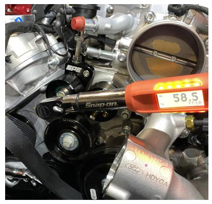
3. Torque Idler pulley bolt to 55-60 LB FT
