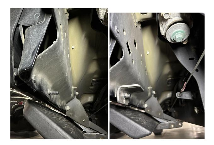
2. Mount the included L bracket on the rear most stud on the body at the pinch weld. We prefer this location on the 17-23 model trucks. The bracket is designed to work with the factory studs making custom locations easier to achieve.
