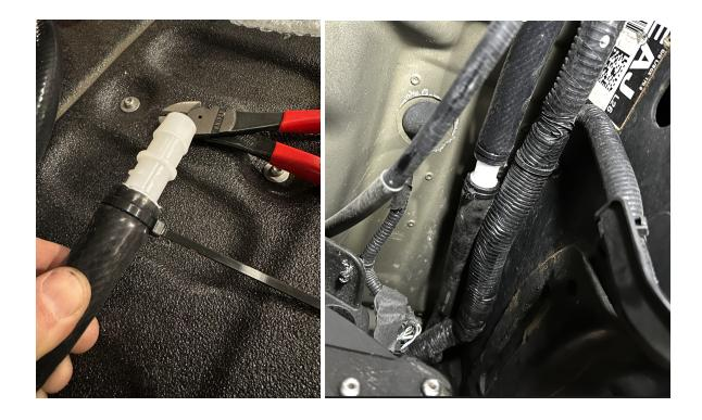
1. Attach the included hose and extension to your existing CCV hose with supplied union and clamps/Ties.
