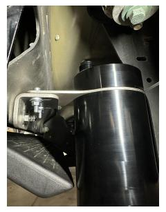
3. Mount the catch can and orientate the drain and hose inlets as shown. Install the catch can to the L bracket with the provided bolts and washers. Adjust and make sure nothing is rubbing.
