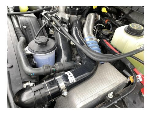
4. Refill cooling system. The air pockets may need to be vented. Get the vehicle to operating temp, allow it to cool, and top off the system.
