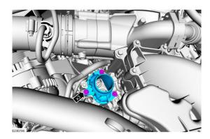
**NOTE:** During installation verify the thermostat vent hole is at the 12 o'clock position..
