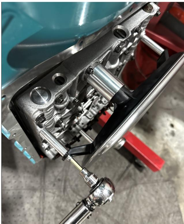
5. Install the filter with the provided extension tube and mounting spacers as shown. Torque the 3 bolts to 100 lb.in (10Nm).
