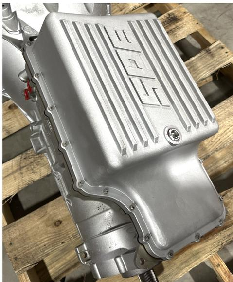
6. Install the SPE transmission pan with the provided 19 M6 bolts. Torque to 100 lb.in (10Nm). Install the drain plug with thread sealant and tighten by hand and add 1-2 full turns.
