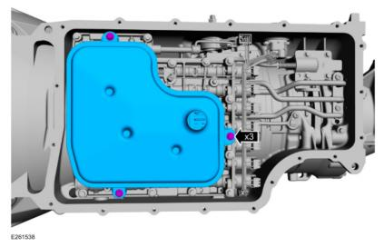
3. With an 8mm socket remove the transmission filter.
