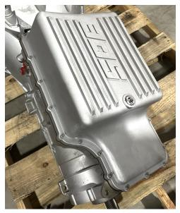
Install the SPE transmission pan with the provided 19 M6 bolts. Torque to 100 lb.in (10Nm). Install the drain plug with thread sealant and tighten by hand and add 1-2 full turns.
