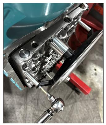
5. Install the filter with the provided extension tube and mounting spacers as shown. Torque the 3 bolts to 100 lb.in (10Nm).
