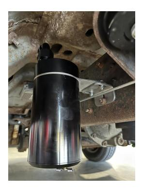
4. Mount the catch can and orientate the drain and hose inlets as shown. Install the catch can to the L bracket with the provided bolts and washers.
