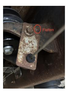
3. Loosen the E-brake cable guide bracket flatten/straighten the locating tab with pliers and reinstall with the bolt loose so that it can be adjusted to keep the cable away from the catch can after installing it.
