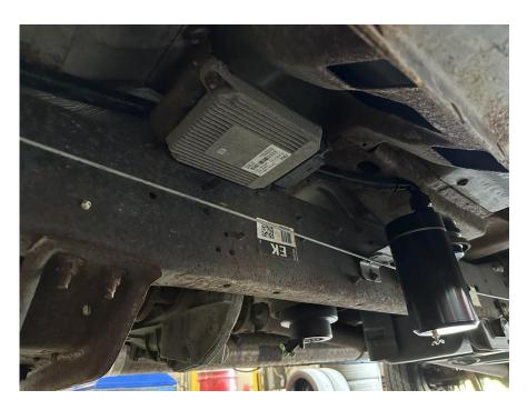
5. Install the 90 degree hose end and route the house similar to the picture above and connect to the hose end by simply pushing it on. No clamp needed. You can now adjust the E brake guide bracket so that its not rubbing the catch can then tighten the bolt.
