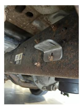
2. Mount the included L bracket on to the closest fuel pump bracket stud closest to the rear of the vehicle as pictured above. We prefer this location on the 11-16 Model trucks. The bracket is designed to work with the frame studs and nuts making custom locations easier to achieve.
