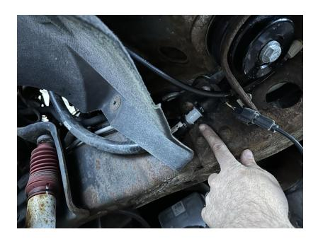
1. Attach the included hose and extension to your existing CCV hose with supplied union and clamps/ties.
