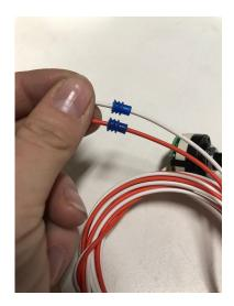
• Insert both wires into the back side of the plug using the blue grommets to cap the opening to prevent any moisture.
