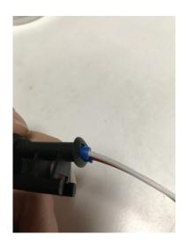
2. Locate the fuel temperature sensor under the hood (drivers side of engine)., disconnect the sensor & plug your EZ Lynk SOTF plug into the disconnected sensor.
