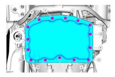
Clean off all the gasket/ silicone from the bottom of the upper oil pan. Install the O ring and drain plug into the SPE Pan. Install the lower oil pan and the bolts.
