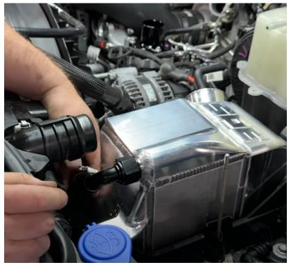
8. For optimum performance, SPE recommends removing the secondary radiator thermostats. This is a free and easy upgrade. The thermostats are located in the secondary radiator end tank(s). Remove the front grill to gain access. Remove the covers to take out the thermostat(s), and then reinstall cover(s). Early models have two, one on each side; later models only have one.
