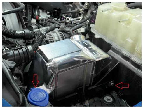
6. Prepare the uppermost intercooler hose to be run to the intercooler. The upper hose will run to the bottom of the SPE intercooler, as shown. Cut and remove the plastic clamp off of the factory hose and remove the hose. Use the supplied hose, hose end, and clamps as shown.
