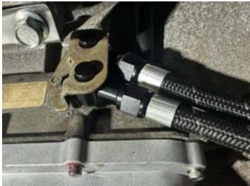
10. Install the new hoses routing them the same as the factory. The longer hose with the 120 degree end will attach to the forwardmost transmission cooler fitting and the top transmission fitting. The shorter hose with the 90 degree end will attach at the cooler (rearmost) and the straight end at the bottom transmission case fitting. Referencing to the images on the next page.
