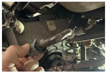
2. Using a Trans cooler disconnect tool, such as the AST 8023, which is designed for  $\frac{1}{2}$  lines, or an equivalent tool, remove the lines from the cooler. Allow them to drain.
