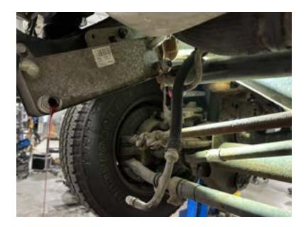
7. Using brake/parts cleaner, clean where the new fittings will go into the transmission case and cooler.
