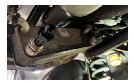
9. Install the provided 4 o-rings onto the transmission case fittings. Lube the o-rings and install the fittings. Reinstall the retaining plate and bolt. Tighten to 18Lb-ft.
