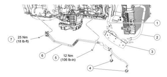
\*\*\*There are multiple ways to remove the transmission lines. We recommend cutting the lines in front of the oil filter housing and removing them in two sections.
