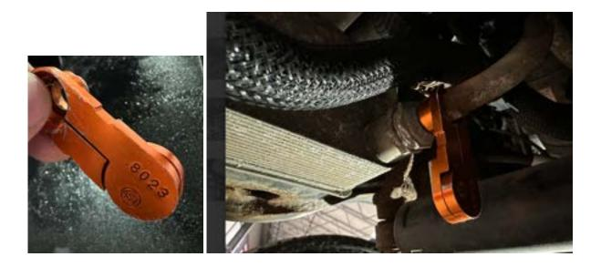
3. Remove the retaining bolt for the OEM line bracket towards the front of the engine.
