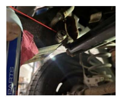
8. Using a light grease or transmission fluid, lube and Insert the fittings into the cooler, pushing until you hear an audible click. Verify by pulling outward on the fittings making sure they are installed properly. Reinstall the plastic clips.
