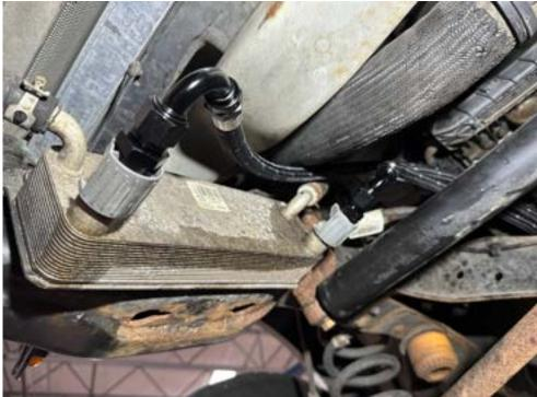
11. Make sure all of the AN fittings are tight. Use the provided zip ties as you see fit to make sure the lines are routed correctly away from sharp objects. Start the vehicle, get it to operating temperature, and top off the transmission with Mercon LV or equivalent fluid.
