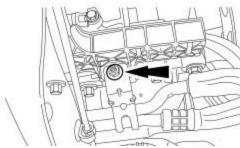
4. Remove the retaining bolt where the lines attach to the transmission case. Using a screwdriver and sidecuts, remove the push clips that hold the retaining plate to the lines as shown.
