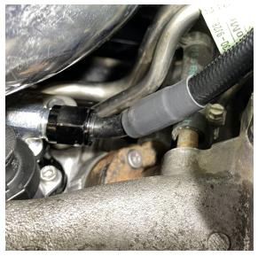
10. Teflon tape and install the fittings into the Fuel manifold as shown below.
