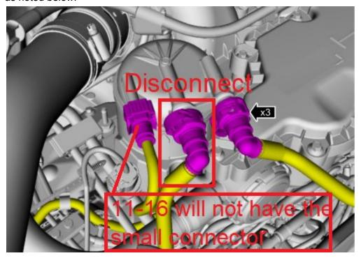
3. With the top of the cp4 now accessible remove the Volume Control Valve (MPROP) Be sure to take note of the tightness.
