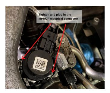
9. Screw on the 45 degree end of the supplied premade hose tighten with the fitting pointing up.
