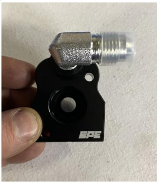
7. Install the 2 supplied o rings on the base of the adapter. After making sure the bore of the pump is clean push the adapter in until seated flat in the pump.
