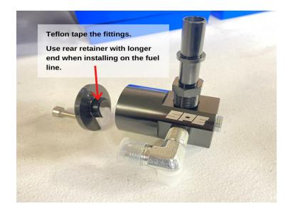
11. Install the fuel manifold on the fuel line as shown using the taller of the two included retaining washers and included M6 allen bolt. Tighten premade hose nut, and install the quick disconnect hose to the fuel filter and manifold.
