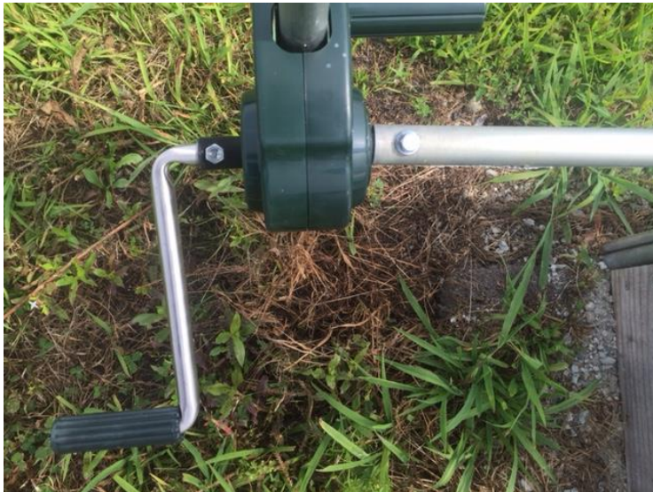
Photo: Fully attached winch to 3/4" EMT conduit.
