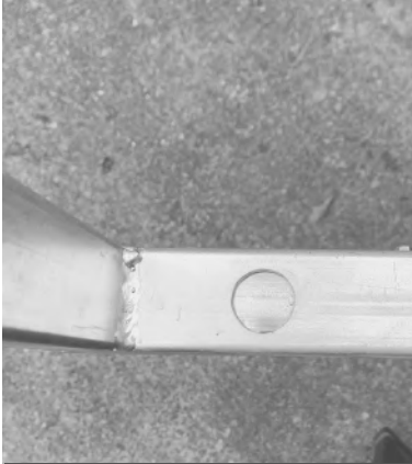
Door Frame Corner with vertical bar installed
