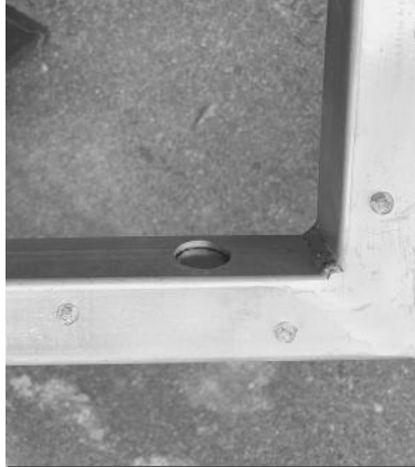
Door Frame Corner back side view with #8 self-tap screws. Showing wide opening
