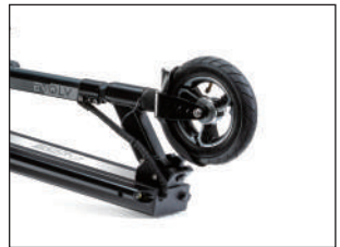
Step 6: Lift the folding lever and push the steering column forward at the same time to release the folding mechanism. While holding down the lever, fold the steering column down towards the deck until it locks into position.
