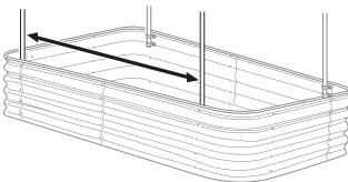
Preassemble two 90--Degree Connectors by inserting the bolt from the outside and the nut on the inside. Be sure to have the flange on the nut facing into the connector.
