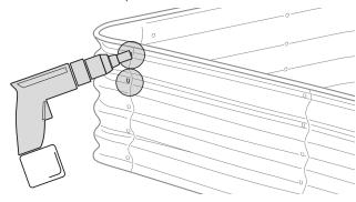
On the INSIDE of the bed, install the One Hole Straps into the top two holes using the hardware you removed in Step 2. Orient the strap, so the loop is closest to the end. Finger tighten the nuts..
