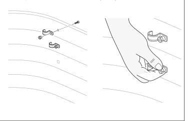
Insert the vertical support down through both One Hole Straps, so the bottom of the conduit is flush with the lower One Hole Strap. Hold the vertical support in place while you tighten the nut.
