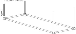
Tighten all of the bolts using the Allen key and adjustable wrench.
