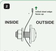
Attach all nuts loosely & then tighten using a screwdriver or cordless drill. Failure to tighten each nut and bolt to its maximum may cause failure.
