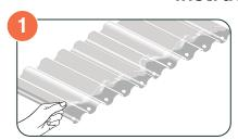
Peel protective plastic 1 inch past the punched holes. Remove remaining plastic once fully assembled.
