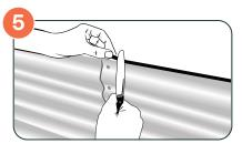
Remove the remaining protective plastic. Starting on a straight length of steel, push the safety edge over the rolled steel edge. Where the steel panels join using a butter knife to pry open will assist in attaching. IMPORTANT: Ensure the safety edge starts and finishes on a straight section of steel, preventing detachment.
