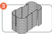
Assemble all side panels first and then attach to the corner sections. Ensure that you attach the corners on the outside of the straight sheets.
