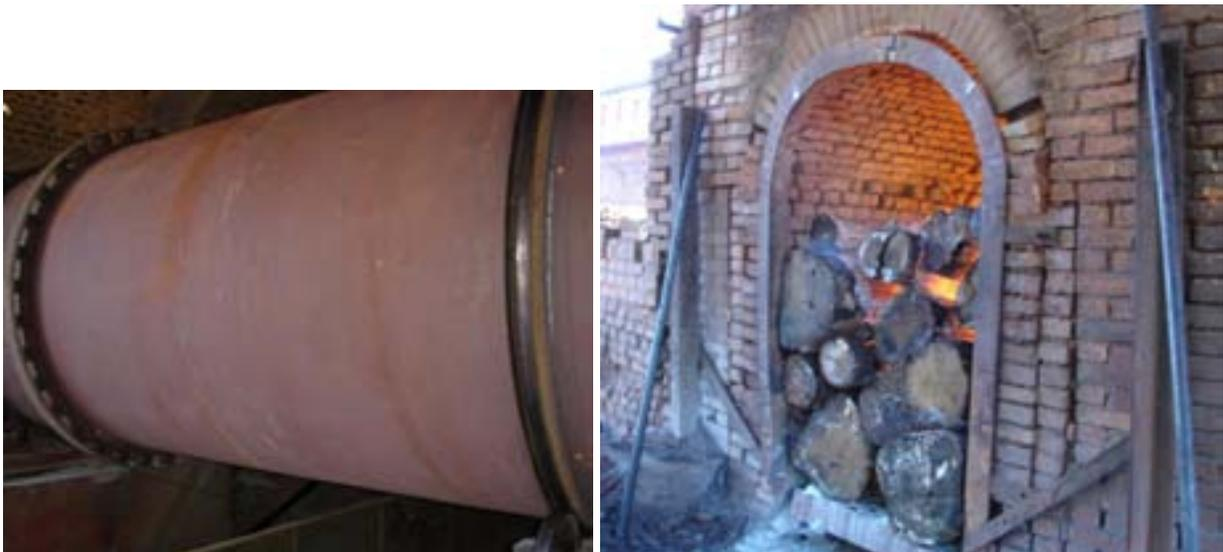
Picture 6. The *secadero* (left) which dries the yerba mate leaves with hot air and the wood-burning oven (right) that supplies hot air to the *secadero*.
