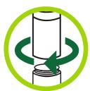
Unscrew the mouthpiece from the heating chamber.
