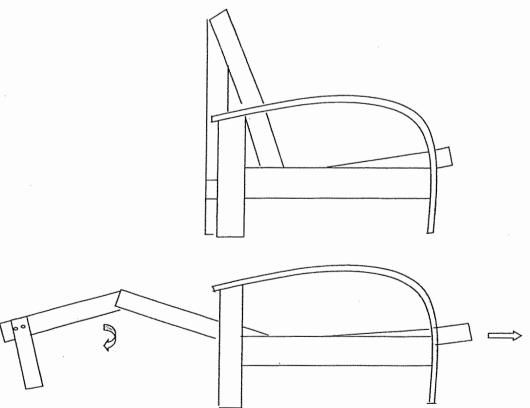
To convert into bed: Pull the rear deck gently down and then pull the front deck forward until it stops. To convert back to lounge position, push the front deck inward and then lift the middle deck upward and push the rear deck toward the back of the arm.
