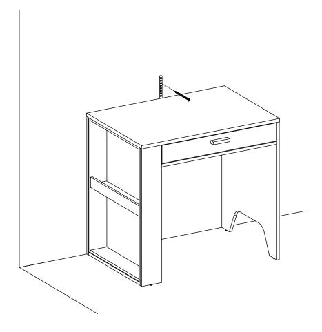
We strongly recommend that this product is permanently fixed to the wall or other suitable surface. Seek advice from a qualified trades person on how to attach this wall strap to your specific wall.
