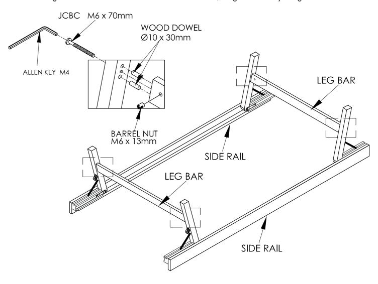
**STEP 3**Attach the End Panels to the Side Rails with Bolts and Barrel Nuts, using the Allen Key to tighten.
