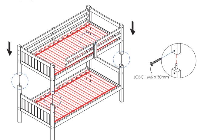
**STEP 3**Attach the Support Rail to the Headboard and Footboard using the Bolts and Barrel Nuts with the Allen Key.
