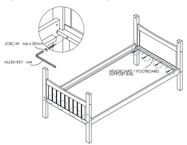
**STEP 4**Lay the Slats, then using the JCBC-W M6 X 30mm Bolts, attach these to the Side Rail.
