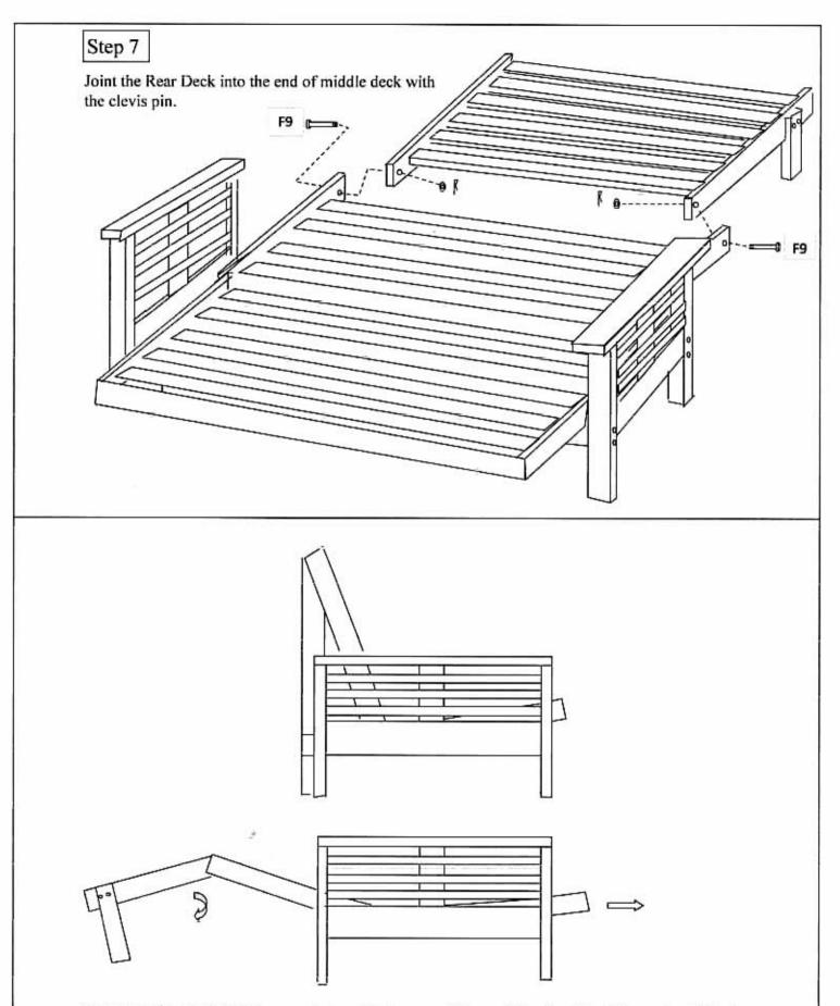
To convert into bed: Pull the rear deck gently down and then pull the front deck forward until it stops. To convert back to lounge position, push the front deck inward and then lift the middle deck upward and push the rear deck toward the back of the arm.
