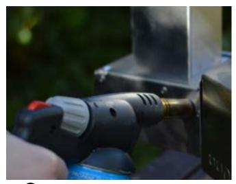
4 If lighting using a blow torch, point the flame through the hole on the side of your burner. Hold it here for 30-45 seconds or until your pellets are alight.
