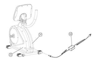
4. Insert Plug Cord (No.59) and AC Adapter (No.60) into the frame.
