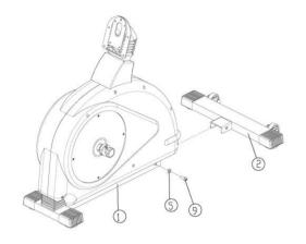
1. Attach the rear support tube (No. 2) to the frame using the Flat Washer (No.5) and Hex Screw M8\*20 (No. 9).
