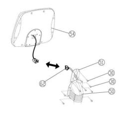
2. Attach the display (No.54) to the display mount by using the screws. Connect the display in by feeding the control wire (No.62) through the center hole in the display mount.
