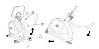
3. Handle Assembly: Insert the Handle (No.11) to the main frame and fixed by Locking Pin (No.10) for Transportation or Storage purpose. Simply remove the locking pin to rotate the handle in and out of storage mode
