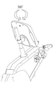
The display rotates 360 degrees for adjusted viewing angles. Use the easy release clip to adjust the display up and down as well as swivel.
