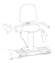
Pull up on the yellow, horizontal seat handle, and swivel to rotate the seat right or left, up to 90 degrees. Release the handle to lock into position.
