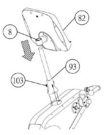
Attach the Display post (93) to the PhysioMax using 3 of the M5 screws (103). Slide the Display (82) onto the Display post (8), and tighten the screws.
