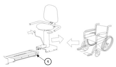
Remove the two rubber stoppers located on each side of the seat rail (1). Pull back on the seat adjustment lever to adjust the seat position. Continue to slide the seat off the rail to allow for wheel chair access.
