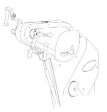
Pull out the black knob to adjust the crank arm length, there are 3 positions. Be sure to hold onto the handle so the arm does not drop.
