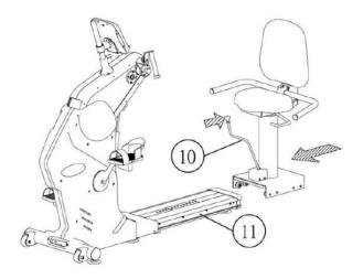
Pull back and hold the Movement Lever (10) then slide the entire assembly forward into the seat-rail, making sure the rollers are moving smoothly within the Aluminum rail (11).
