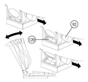
Pull out the back seat knob to adjust the angle of seat back. (1-3)
