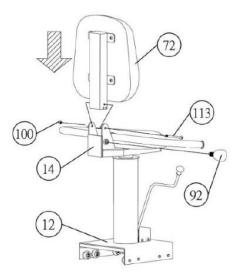
Insert the seat back support frame (14) that is connected to the seat back (72) into the seat base frame (12). Using the bolt (113) and the nut (100) secure in place.
