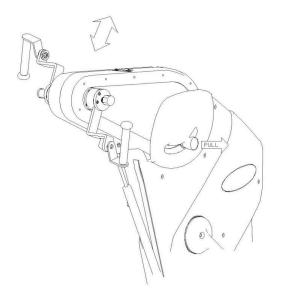
Pull out the orange knob to adjust the arm crank height and positioning, there are multiple angle settings. Lock into place by releasing the orange knob and tightening.
