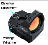
The Elevation and Windage turrets allow for 40 MOA per revolution. Each adjustment click moves the reticle 1 MOA.
