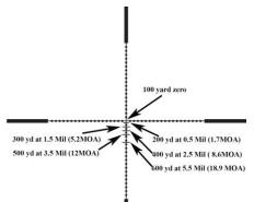
The true Mil relationship is at 4X. On lower vertical portion there are also five BDC hold over lines, which will be used at 4X. After you zero the scope at 100 yards, the 1<sup>st</sup> BDC line is for 200 yard shot. The 2<sup>nd</sup> line is for 300 yards. The 3<sup>rd</sup> BDC line is for 400 yards. The 4<sup>th</sup> BDC is for 500 yards. The 5<sup>th</sup> BDC
