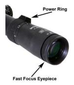
Hold the scope about three to four inches from your eye and look through the eyepiece at a featureless flatly lit bright area such as a wall or open sky. If the reticle is not sharply defined instantly, you just need to turn the fast focus eyepiece inwards or outwards until the reticle appears in sharp focus.
