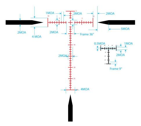
The center of the HR1 reticle has a 2 MOA by 2 MOA cross. The opening in the center of the reticle is used to frame and range a known size 36" target.
