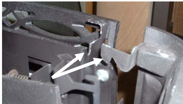
Photo 9 – Front Panel Mounting Tang Detail
