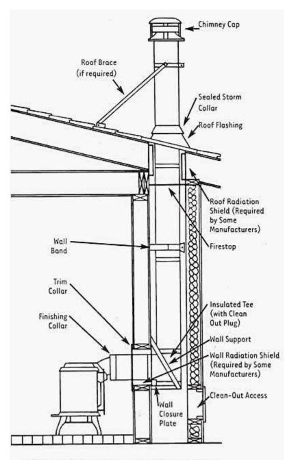
Through-the-Wall Installation — Factory-Built Chimney
