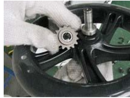
8. Rotated to remove the both right and left flywheel.
